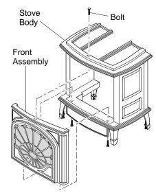
Figure 13 - Removing Front Assembly
